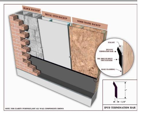
When the flashing material is terminated in a vertical condition, the IPCO Termination Bar should be used and caulked at the top edge. Install the termination bar with concrete screws or other mechanical fastening devices. Place the bent portion of the termination bar just above the top edge of the flashing being secured (see detail inset above).
