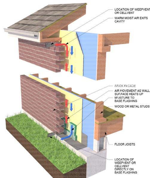
Use WeepVent to increase ventilation at the top and bottom of wall
